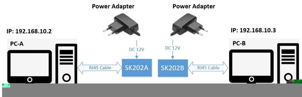
Figure 6. Iperf3 test Schematic diagram with SK202
